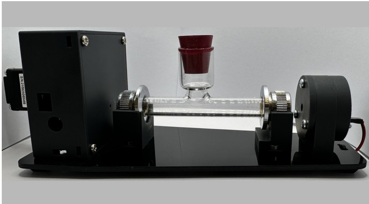
Fig.5 The PicoPOL Optical Bench – Detector module at left, Source module at right and two cell carrier blocks in between.
